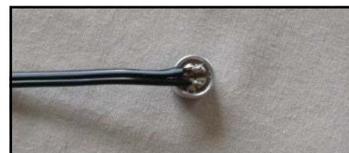
Fig. 6: Lead soldered to mic terminals.
