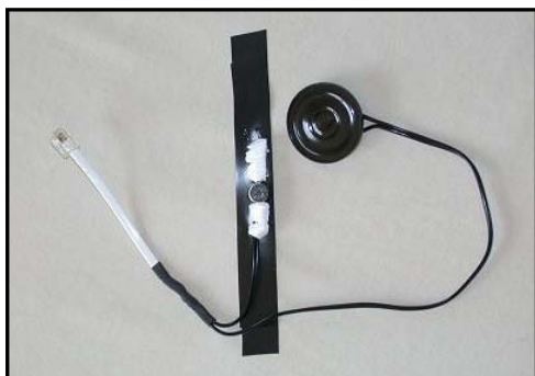
Fig. 7: Mic element glued to tape.
