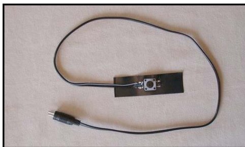
Fig. 12: Switch glued to electrical tape.
